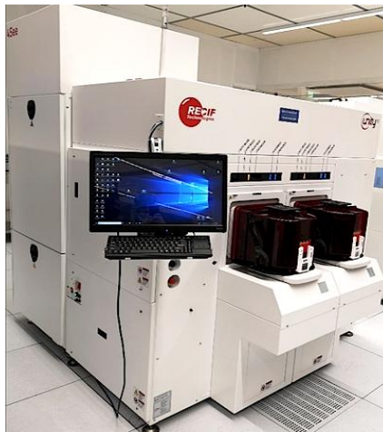
RECIF 300mm equipment with Unity inspection module
